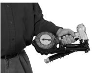
Slide caps along the feed chute with fingers until they engage the cap feeder. Pull the cap feeder back and release to advance caps until the first cap is under the nose of the tool.
