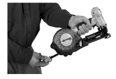
Depress the latch on the staple follower and pull back. Insert two staple strips. Slide staple follower in and secure.
